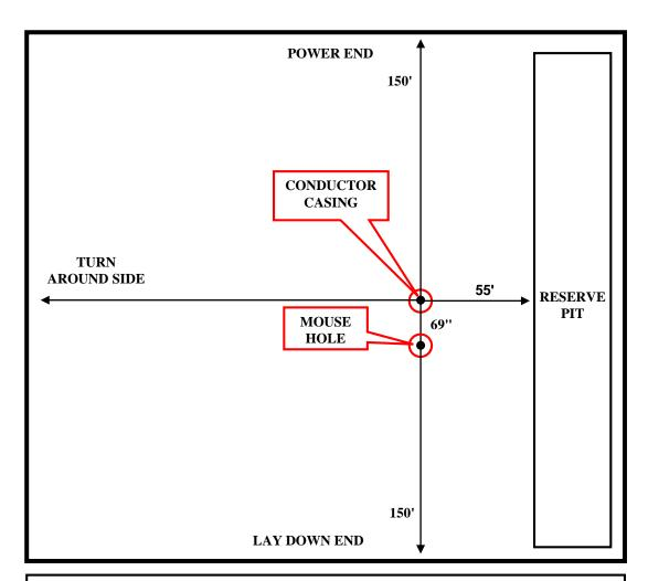
**Note:** <u>All</u> measurements are from the center of the conductor casing. The mouse hole is 69" from the center of the conductor casing w/0° slope (angle). This rig has a top drive so the mouse hole should be a minimum of 75' deep (from ground level) with casing or liner with a minimum ID of 10". The reserve pit is a minimum of 55' from the center of conductor casing.
