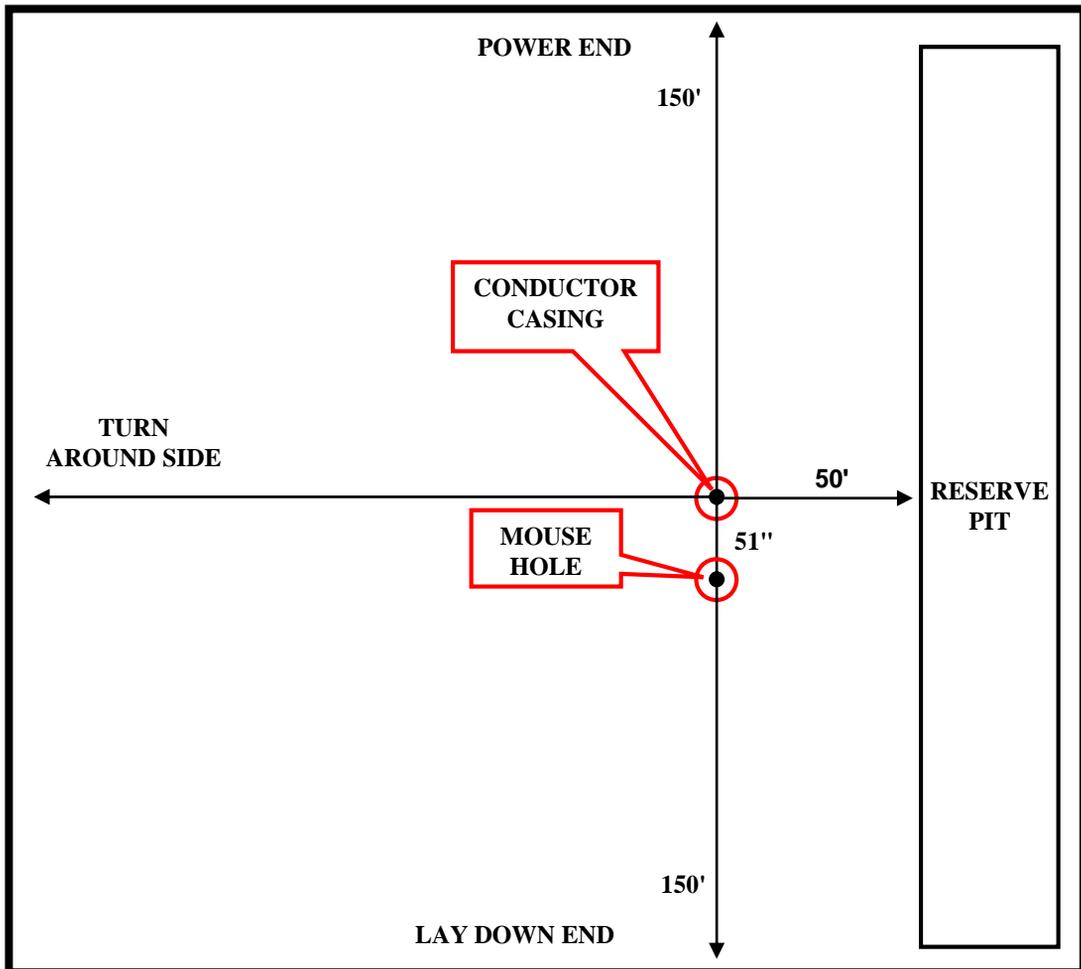
**Note:** All measurements are from the center of the conductor casing. The mouse hole is 51" from the center of the conductor casing w/ 0° slope (angle). This rig has a top drive so the mouse hole should be a minimum of 75' deep (from ground level) with casing or liner with a minimum ID of 10". The reserve pit is a minimum of 50' from the center of conductor casing.
