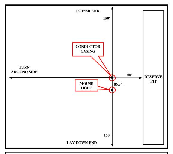
**Note:** <u>All</u> measurements are from the center of the conductor casing. The mouse hole is 86.5" from the center of the conductor casing w/  $0^{\circ}$  slope (Angle). This rig has a top drive so the mouse hole should be a minimum of 75' deep (from ground level) with casing or liner with a minimum ID of 10". The reserve pit is a minimum of 50' from the center of conductor casing.
